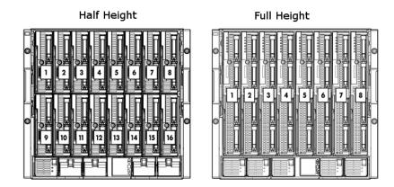
The number of fans in the enclosure influences the placement of the server blades. Use the following table and the numbering scheme in Figure 1-3 to determine the placement of the server blades in the enclosure, based on the number of fans.
